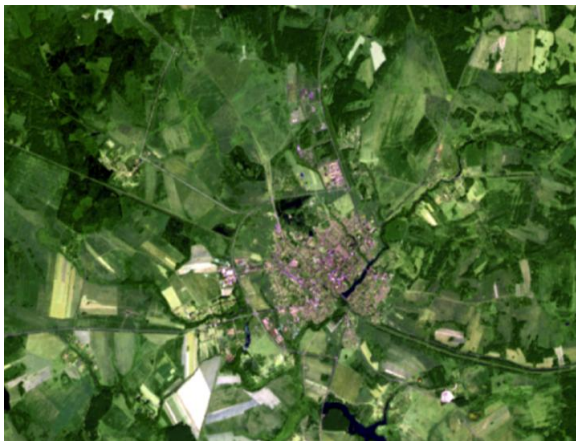
A raster image of a part of the territory of Mogilev region, obtained by combining the RGB channels of satellite Landsat-8
