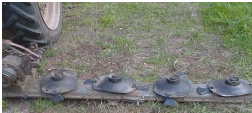
Fig. 3. Multi-rotor mower, equipped with cutting device with trapezoidal knives
